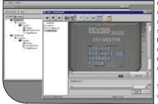
mark, incomplete characters, character voids, incorrect characters, wrong mark, doublestruck mark, smeared mark, blurred mark, scratched mark, character breaks, low-contrast marks, over print, under print and mark orientation.
