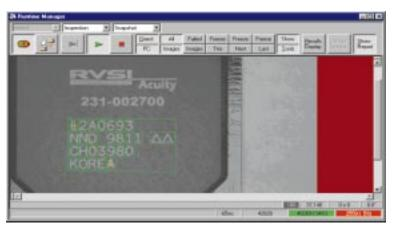
The Visionscape<sup>™</sup> Mark Inspection system offers a built-in Windows<sup>®</sup> NT/95 Graphical User Interface (GUI) for point and click mark training, parameter setting and run-time inspection monitoring.
