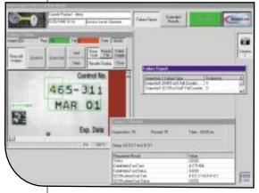
ing normal print variation. Proven OCV (Optical Character Verification) algorithms adapt to acceptable changes in preprinted or overprinted codes to reduce false rejects. Special attention is paid to characters in which a subtle defect might cause it to be mistaken for a different character such as an "O" vs. "D" or "B" vs. "8".
